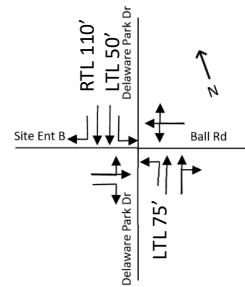
Based on DelDOT's *Development Coordination Manual*, the recommended minimum storage length (excluding taper) of the northbound left turn lane is 75 feet, the southbound left turn lane is 50 feet, and the southbound right turn lane is 110 feet. The projected queues from the traffic analysis can be accommodated within the recommended storage lengths.
